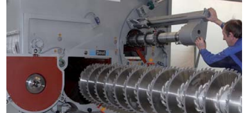
Fig. 6: Simple change of the top and bottom saw shaft
